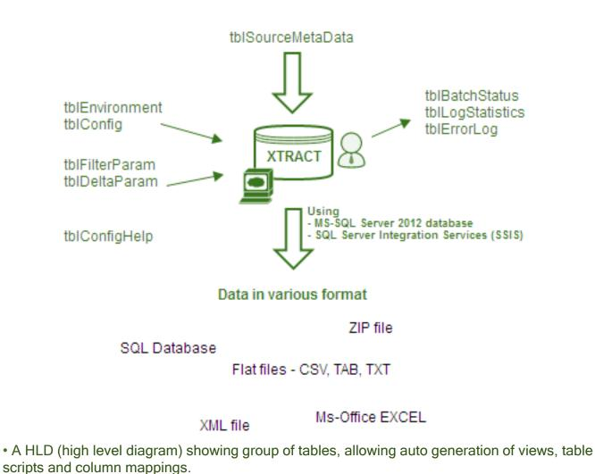
• Repository database holding table configuration, environment, batch & log status, error log, delta-load and data-filter.
